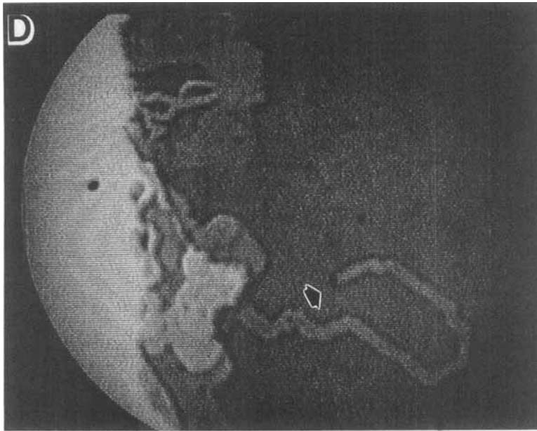
FIGURE 4A - D Sequence showing the propagation of channels across the basal plane surface of graphite by platinum-iridium particles at 1030°C in 5.0 Torr oxygen. Time interval between each frame is 10 sec. (reprinted with permission from Academic Press, Ref. 34).
